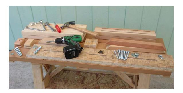
Here are all the parts that go into a **LEVEL-it®** along with a selection of tools to complete the assembly. While a **LEVEL-it®** can be assembled with just hammer, screw driver and some kind of wrench, we are showing both manual and power drivers and several kinds of wrenches. Use the kind of driver and the kind of wrench that you have.
