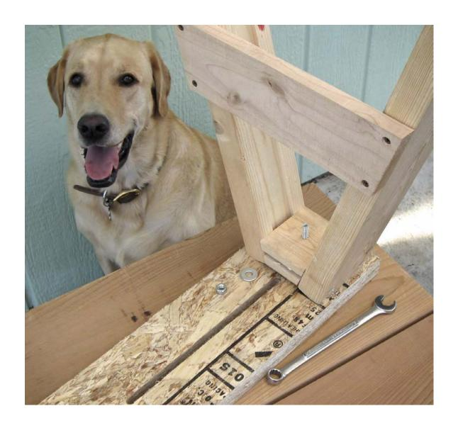
Thread a  $\frac{5}{6}$  X  $3\frac{1}{2}$  carriage bolt through the counterbored holes in the **LEVEL-it**® top and through the holes in the middles of the upper braces...
