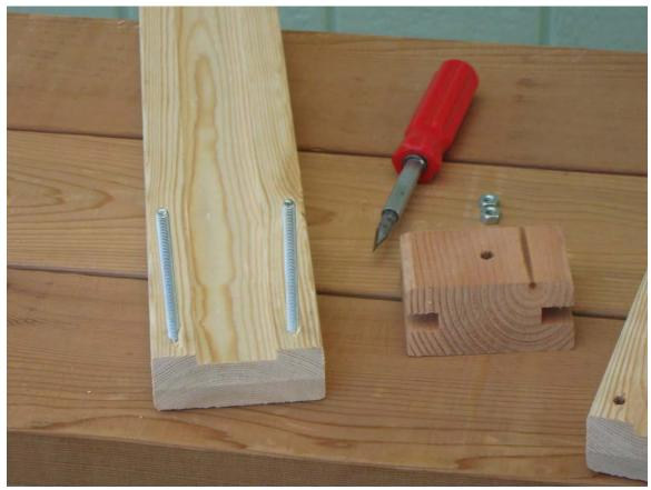
Above is shown a leg with two ¼"X 5" machine screws properly threaded through it.
