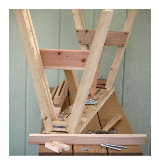
Now that the leg assemblies and diagonal braces have been assembled we can fit the four leg extensions into the grooves of the legs using 5/16" X 3½" carriage bolts, 5/16" fender washers and the large wood wingnuts.
