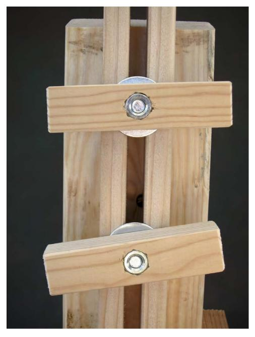
Here is how it should look when the extension is installed in the groove of the leg using two 5/16" X 3½" carriage bolts, two 5/16" fender washers and two wood wingnuts.
