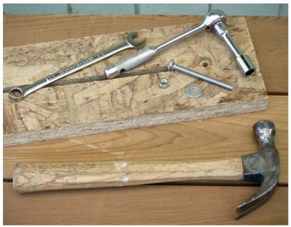
Each leg assembly is attached to the lower side of the **LEVEL-it**® top with a 5/16" X 3½" carriage bolt, a 5/16" flat washer and a 5/16" hex nut. You may need a hammer to gently tap the carriage bolts through the counterbored holes in the **LEVEL-it**® top. You will need some kind of wrench to tighten the nuts onto the carriage bolts. Two kinds of wrenches are shown here. Use the kind you have.
