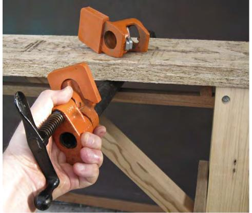
Remove the sliding jaw from a ¾" pipe clamp and slide the pipe between the **CLAMP-it**<sup>™</sup> and the underside of the **LEVEL-it**<sup>®</sup> top as in the photo above. Then replace the sliding jaw onto the ¾" pipe clamp.
