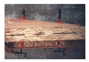
Here is an irregularly shaped object clamped to the edge of a **LEVEL-it**<sup>®</sup> top with two pipe clamps.
