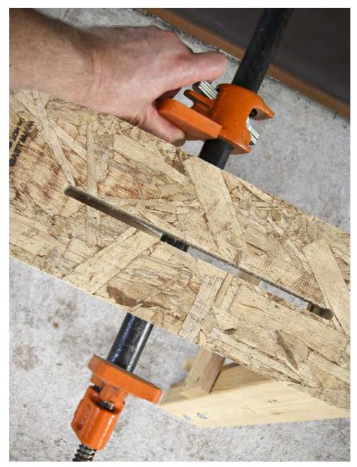
Looking down on the **LEVEL-it**<sup>®</sup> top as the sliding jaw is being replaced onto the pipe clamp should look about like this photo.
