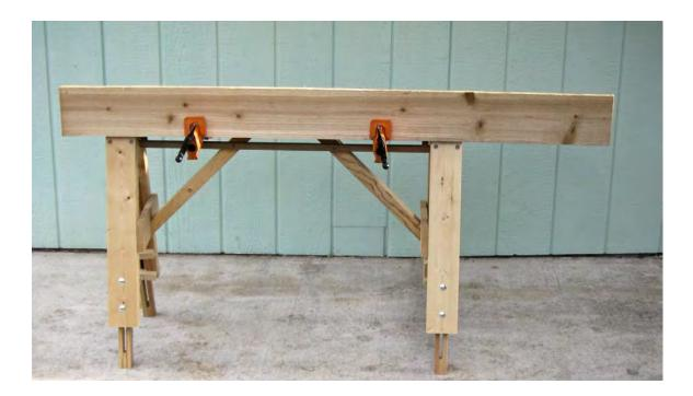
Here is a **LEVEL**-it<sup>®</sup> with a **CLAMP**-it<sup>™</sup>. There are two pipe clamps being held in place by the **CLAMP**-it<sup>™</sup>. Those pipe clamps are holding a board against an edge of the **LEVEL**-it<sup>®</sup> top so that work can be done on the board.
