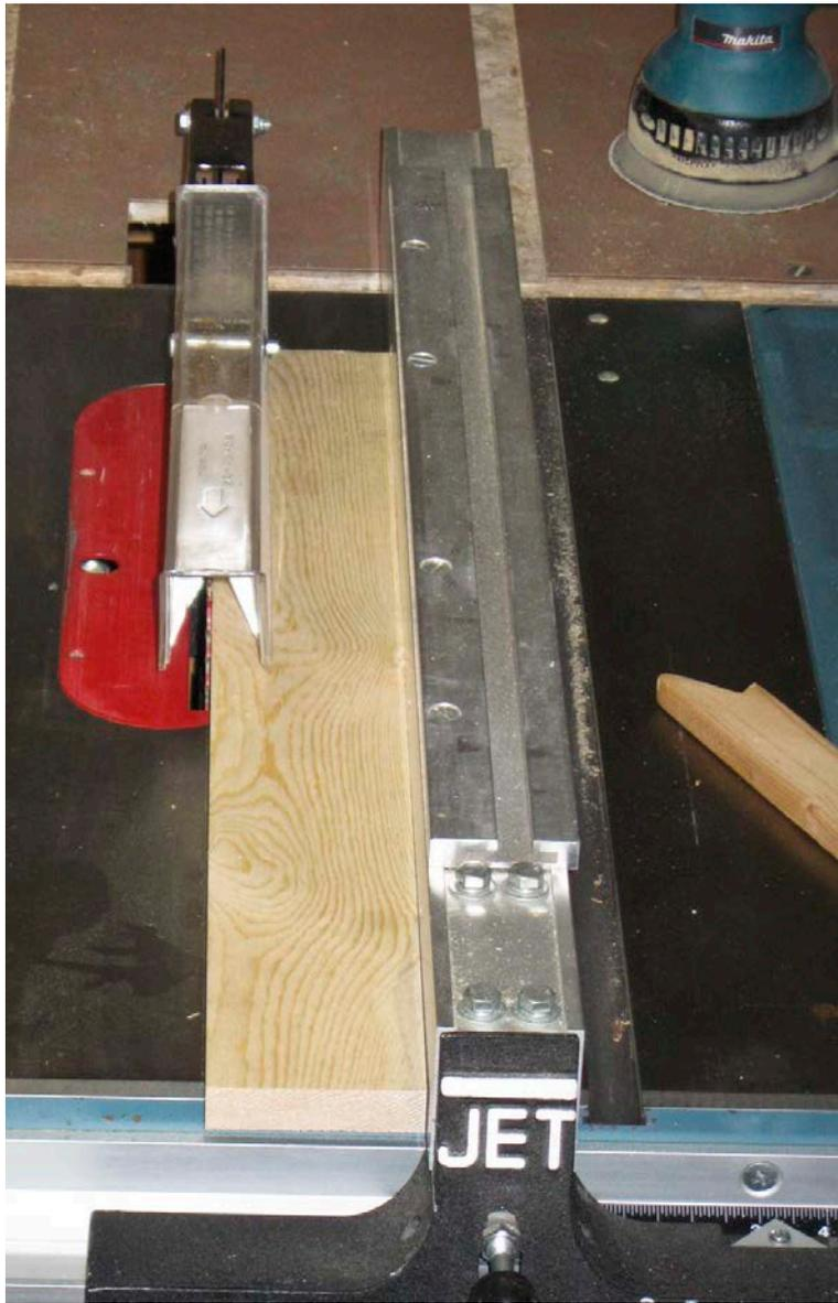
A table saw is the best tool to rip some boards to the proper width to make frame or web pieces. Rip the boards to the proper width as determined by the measurement in the previous step.
