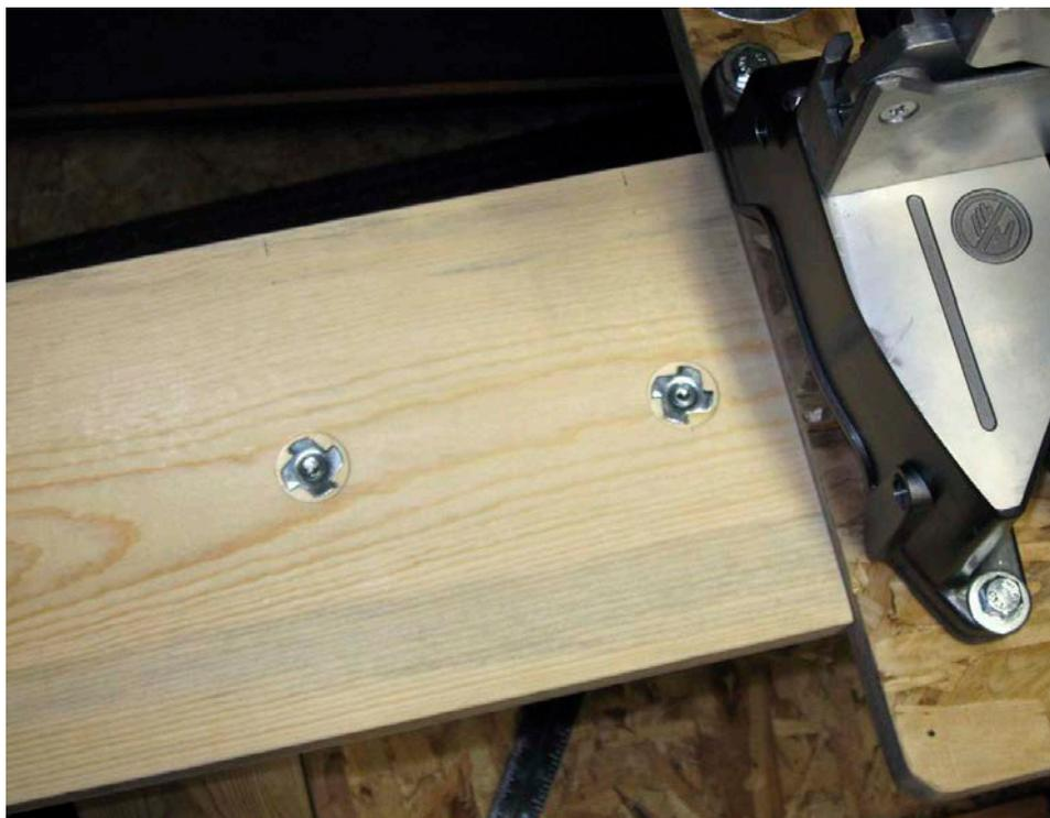
Drill two pilot holes which are the proper size for the Tee-Nuts you will be using. We recommend  $\frac{5}{16}$ ” Tee-Nuts.  $\frac{5}{16}$ ” is the bolt diameter for which the slots in the **LEVEL-it**<sup>®</sup> top are designed. Go ahead and bolt this lower or “base” board securely to the **LEVEL-it**<sup>®</sup> top as shown here.
