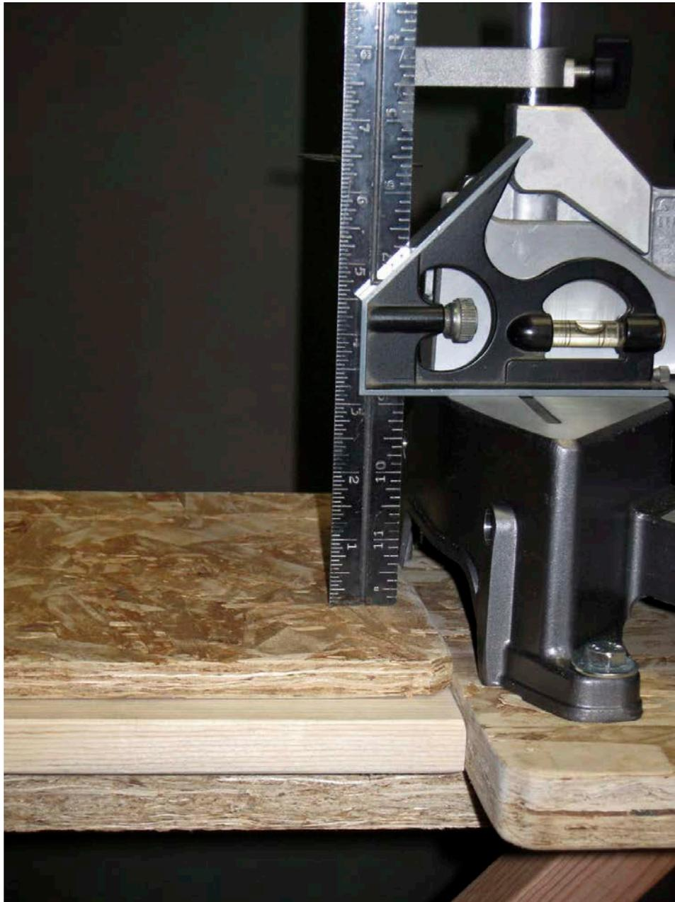
With the lower or “base” board still bolted to the **LEVEL-it**® top, lay the upper board on top of it as shown in this photo. Use a combination square as shown to measure the distance from the surface of the chop saw table to the upper board laying on top of the lower or “base” board. This measurement is the width of the boards that will be used to make the frame or web pieces.
