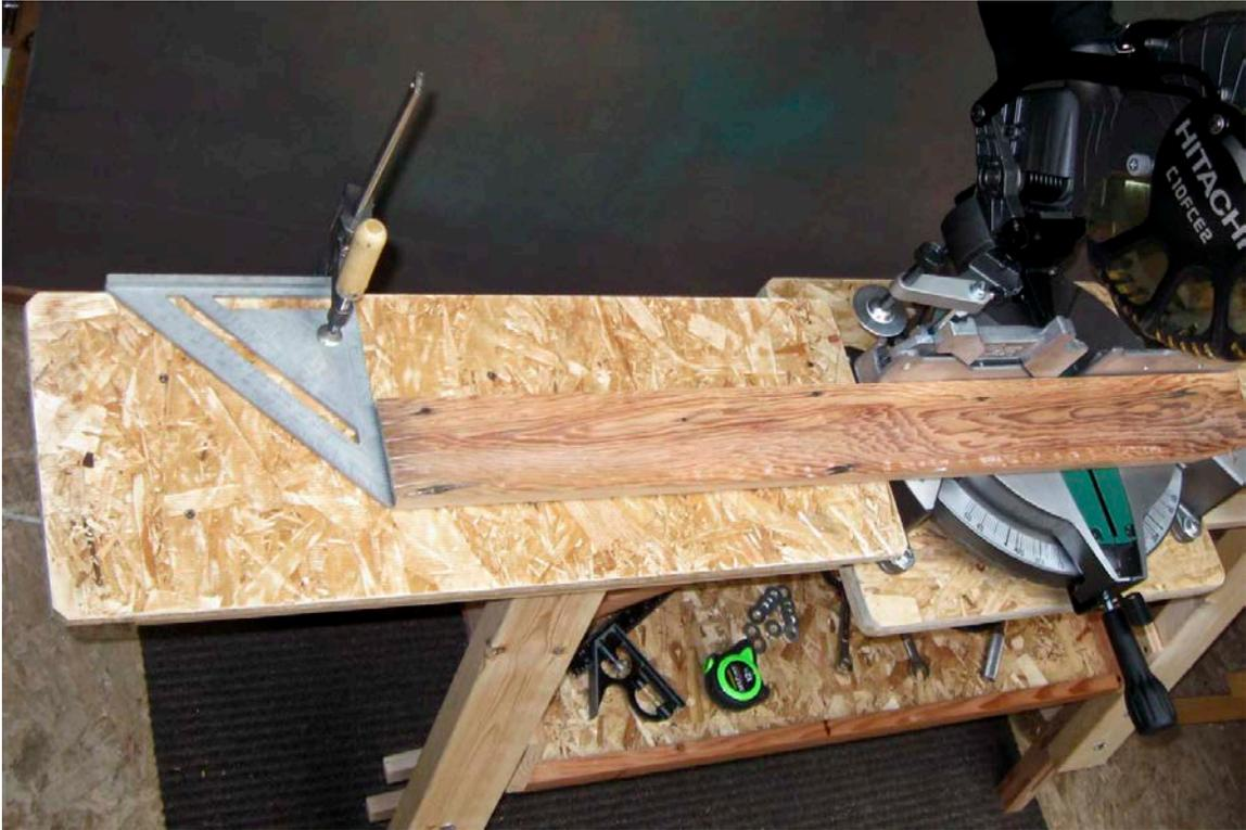
The photo above shows a 6-inch rafter angle square clamped to the edge of the upper board of the extension with a bar clamp. This makes an effective, adjustable stop for repetitive cuts with the chop saw.
