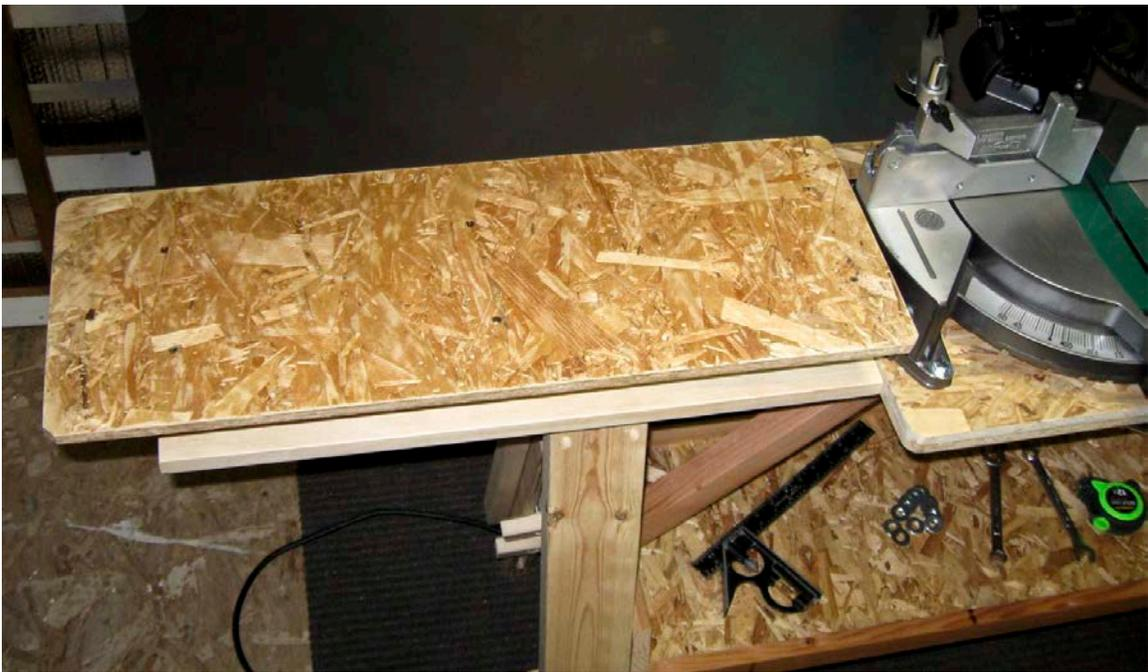
After you have fastened the lower or “base” board and the upper board to the frame or web you can attach your new extension to the **LEVEL-it**® top with two bolts. It should look about like this. Then make the other extension the same way you made the first one and attach it to the **LEVEL-it**® top on the other side of the chop saw in the same manner.
