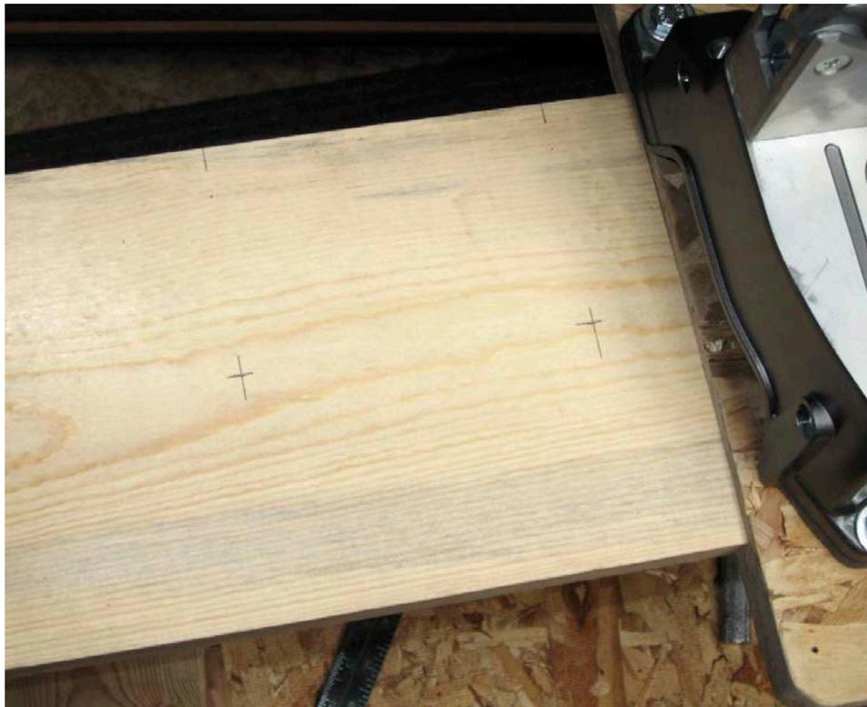
Using a 6-inch rafter angle square or a combination square transfer the marks to the center of the lower or “base” board as shown here.
