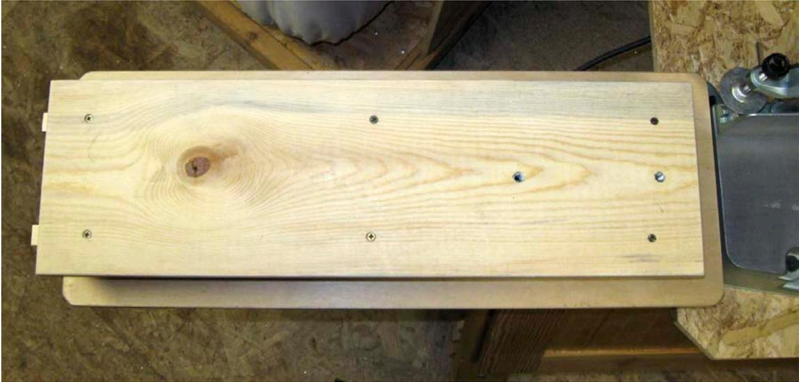
We use screws to fasten the lower or “base” board and the upper board to the frame or web. It makes it easier to take it apart later if we need to replace the upper board due to wear and/or abuse. This photo shows the underside of the lower or “base” board with all the fasteners in place. You can also see the two Tee-Nuts by which this extension is attached to the **LEVEL-it**® top with two bolts.
