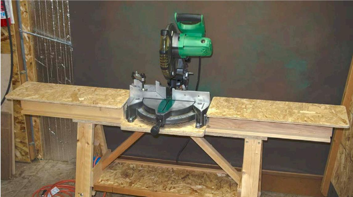
These extensions are made using torsion box construction. They are extremely strong yet easy and inexpensive to make. Additionally there is enough of a lip around the tops of these extensions that you can clamp all sorts of items to them. This makes for a very strong and versatile bench that's almost 6 feet long. The extensions we use in our own shop are between 9" - 9¾" wide.
