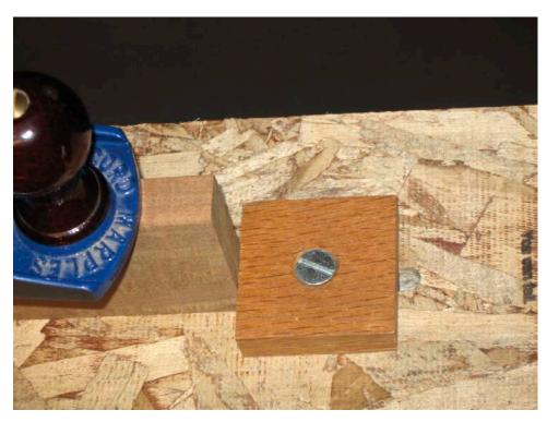
Here a handplane is in use planing the edge of a board using the **DOG-it**<sup>™</sup> to hold the board in place.
