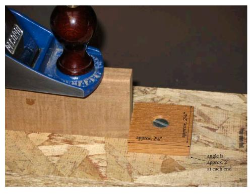
A **DOG-it**<sup>TM</sup> is simply a small, thin piece of hardwood (oak, maple, hickory, etc.) cut to the approximate size shown with slight angles at each of the two ends. A thickness of no more than ½" is recommended.
