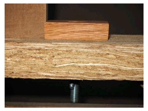
The **DOG-it**<sup>TM</sup> is attached to the **LEVEL-it**® top with a 5/16" X 2½" flat-head machine screw which is countersunk into the top of the **DOG-it**<sup>TM</sup> so that the head of the machine screw does not protrude and damage any tool you might be using. Use a large wingnut and washer to tighten the **DOG-it**<sup>TM</sup> from the underside of the **LEVEL-it**® top.
