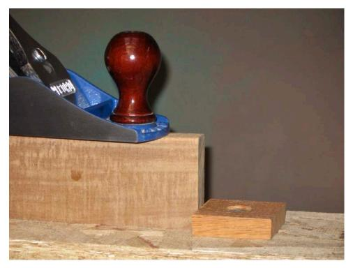
A  $\mathbf{DOG}$ - $\mathbf{it^{TM}}$  bench dog helps to hold workpieces along a workbench top to make it easier to work on them. The slots in the top of a  $\mathbf{LEVEL}$ - $\mathbf{it^{@}}$  make it very easy to position a  $\mathbf{DOG}$ - $\mathbf{it^{TM}}$  anywhere along the length of the top.
