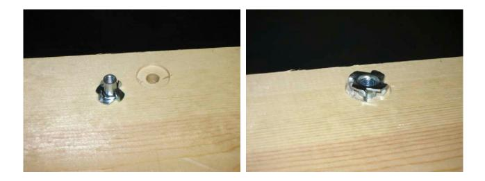
Using the 1" forstner bit, drill a shallow hole only about ½" deep on each of the two marks drawn in the previous step. Next drill a <sup>25</sup>⁄<sub>64</sub>" through-hole at the center of the larger hole. See photos above.
