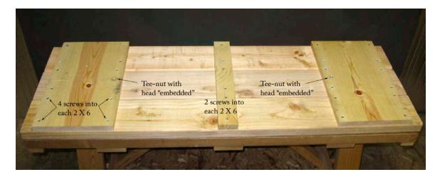
Proceed to screw the 1 X 10's (and the center board) to the underside of the 2 X 6's as shown above. Note that the Tee-nuts are placed so that their large heads are closest to the 2 X 6's — the Tee-nut heads are now "embedded".
