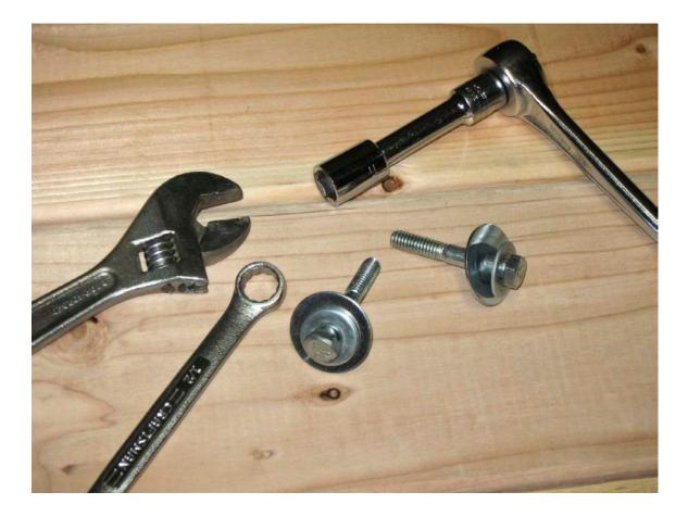
Here are the two <sup>5</sup>⁄<sub>16</sub>" X 2" bolts, each with a flat washer and a fender washer ready to mount the **TOP-it**<sup>™</sup> to the **LEVEL-it**<sup>®</sup>. Tightening of the bolts requires a <sup>1</sup>⁄<sub>2</sub>" or adjustable wrench. Any of the wrenches shown could be used. Pliers are NOT recommended as they ruin the heads of the bolts over time.
