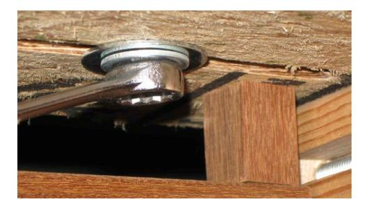
Complete mounting the **TOP-it**<sup>TM</sup> to the **LEVEL-it**<sup>®</sup> by tightening each bolt with a wrench until snug as shown here.
