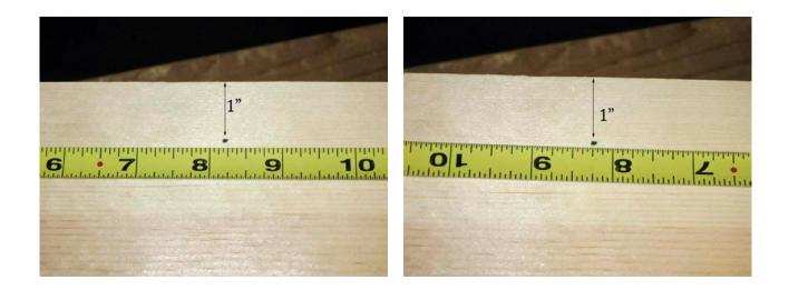
Measure along the lengths of two of the 1 X 10's and place a centered mark 1" from an edge of each board. (By measuring first from one end and then the other the exact center can be found)
