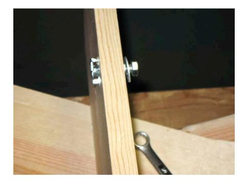
While it is possible to simply tap the Tee-nuts into place with a hammer, using a short bolt and several washers along with a wrench to tighten each Tee-nut into place ensures that they go straight and perpendicular into the holes. This makes the attaching and removing of the **TOP-it**<sup>TM</sup> to and from the **LEVEL-it**<sup>®</sup> much easier every time one bolts or unbolts it.
