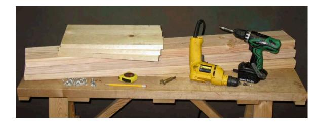
Here are all the parts and tools to make a **TOP-it<sup>TM</sup>** cut and ready to be drilled and assembled. Also needed are 4 shims that will be used to space the 2 X 6 pieces evenly (2 popsicle sticks, each cut in half, work well).
