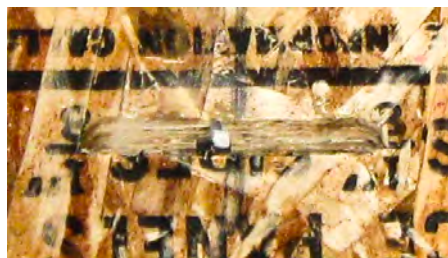
Close up showing router bit cutting slot.
