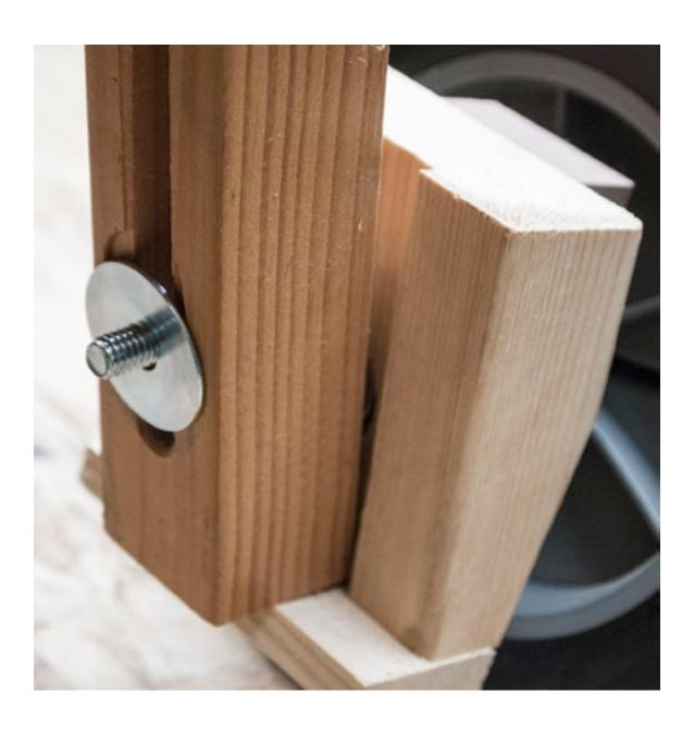
7- Thread a wood wingnut onto the bolt with the metal nut in the wingnut on the outside. Tighten the wingnut until the wheel BRACK- $it^{TM}$  is secure on the leg extension.
