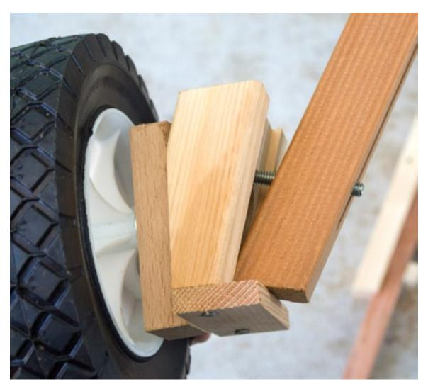
6- Insert a fender washer onto the 5/16" bolt as shown.
