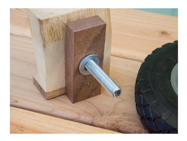
2- Insert the axle/bolt through the axle hole in a wheel hub so that the part of the hub that sticks out a little is touching the washer installed in step 1. Place a second ½" washer over the axle/bolt now that the wheel is on.
