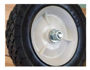
4- Using two wrenches against one another tighten the two ½" jam nuts together so that neither will turn on the axle/bolt and the wheel turns easily on the axle/bolt and does not move in and out very much. Some very slight "play" is OK.
