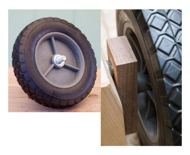
3- Thread a ½"jam nut onto the axle/bolt and tighten it very gently to the point that it contacts the washer. The wheel should turn easily and not move in and out very much. Thread a second ½"jam nut onto the axle/bolt and tighten it to the point that it contacts the first ½"jam nut.
